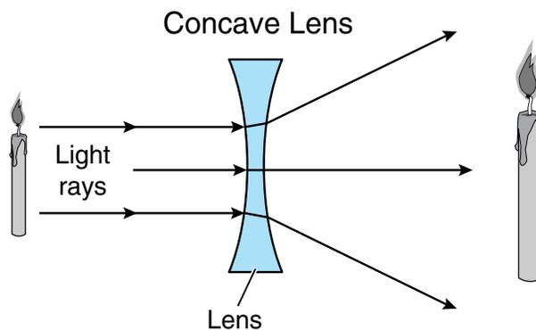
A lens that is thicker at the edges than in the middle bends light rays away from one another.
