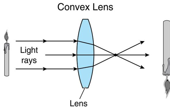
A lens that is thicker in the middle than at the edges bends light rays toward one another. This is the type of lens found in your eye and in a telescope.
