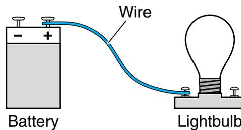
This drawing shows an incomplete circuit. Only one pole of the battery is connected to the lightbulb. Electricity does not move through the wire, and the lightbulb does not light up.
