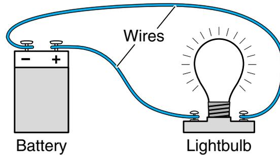
This drawing shows a complete circuit. An electric current moves from one end of the battery to the lightbulb and then back to the other end of the battery. Because the circuit is complete, electricity moves through the wires, and the lightbulb lights up.
